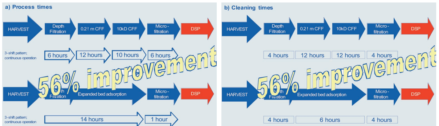
Fig. 2: Improvement in processing and cleaning cycle times driven by the introduction of EBA technology to the manufacturing process for a chimeric protein (Fab + effector molecule)
