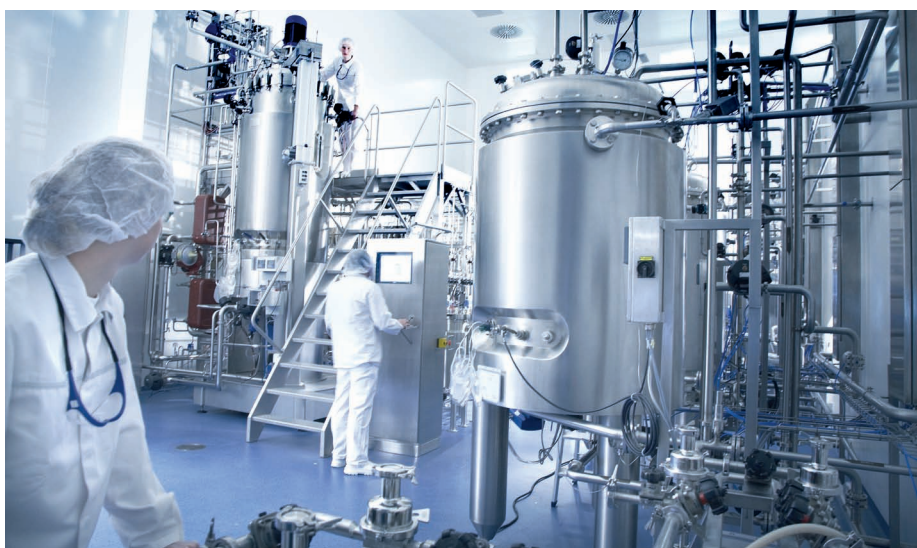
Fig. 3: Upstream processing equipment with a 1.5m 3 fermenter (left) and support tanks at Richter-Helm BioLogics in Bovenau, Germany
